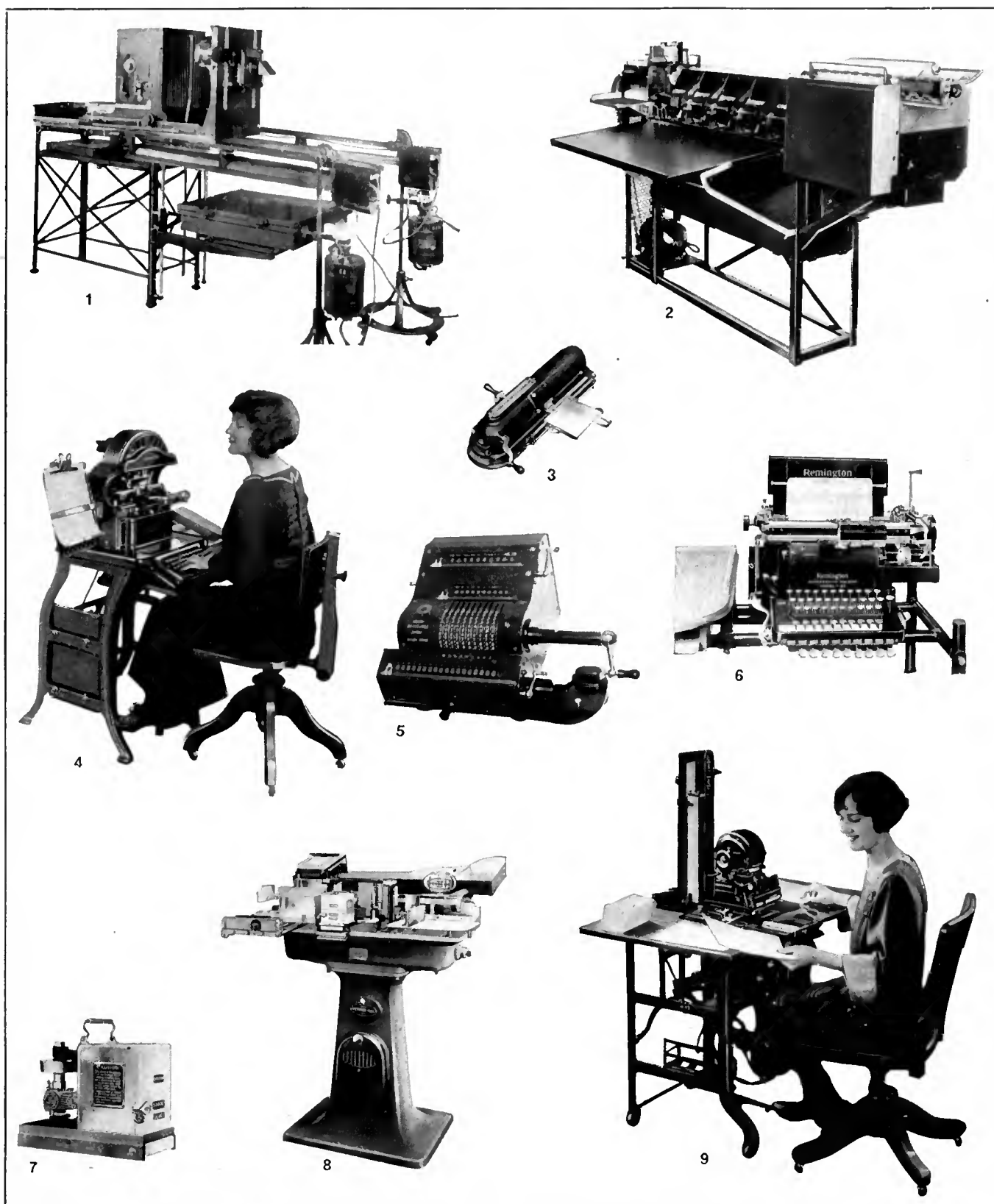
FIG. 1. Photostat. This machine copies photographically any written or printed material, and automatically develops, fixes and washes the photographic copy. A machine used to save the labour of keeping documents. FIG. 2. Electric Printing, Tabulating and Accounting Machine. This machine tabulates data which have been previously sorted on another machine, not shown in illustration, and prints the tabulation automatically on a suitable sized sheet. FIG. 3. The Protectograph. A machine for printing the amount, and at the same time shredding the paper on cheques, to avoid the possibility of forgery. FIG. 4. Graphotype. On this machine, a metal stencil is embossed, which is later used for addressing. FIG. 5. Brunsviga Calculating Machine. FIG. 6. Bookkeeping Machine. Used for posting debit and credit items on ledger sheets. Accounting is balanced with each posting. FIG. 7. Postal Permit Printer. FIG. 8. Postage Meter Machine. A device which seals the envelope and prints indicia which take the place of the ordinary postage stamp. The meter is locked by the postmaster, and postage is paid for the amount shown on the meter. FIG. 9. Addressograph. Prints from metal stencils made by the Graphotype. Addresses envelopes, statements and the like automatically.
