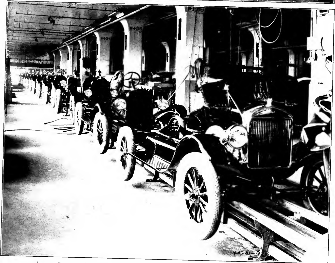
BELOW—Final assembly line in the Highland Park plant of the Ford Motor Company, Detroit. Bodies and chassis having been completed separately, the body is dropped on the chassis as it advances. The chassis in the foreground is just about to receive the body which is seen, slung by chains from the overhead yoke, at the right.
